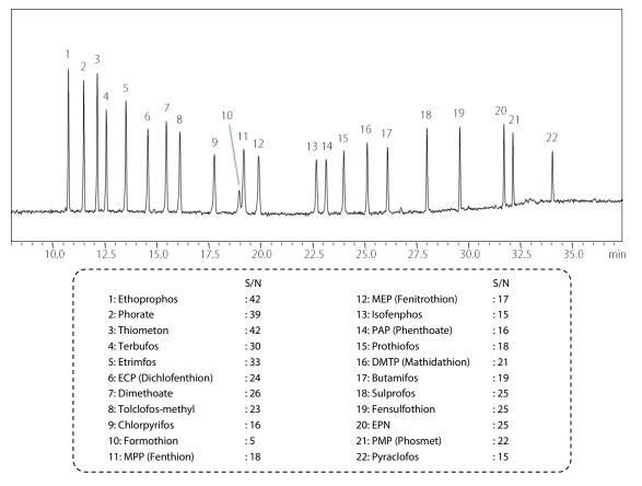
Fig. 2 Chromatogram of Low-Concentration (5  $\mu$ g/L) Organophosphorus Pesticides
