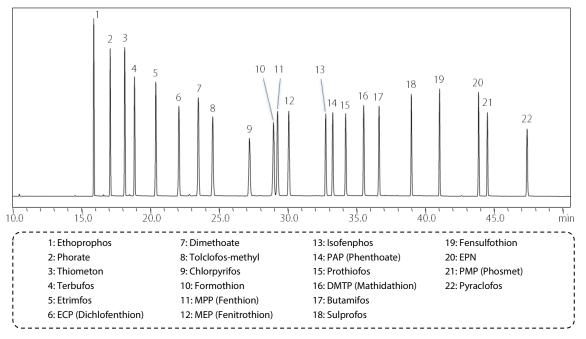
Fig. 1 Chromatogram of 20 mg/L Organophosphorus Pesticides
