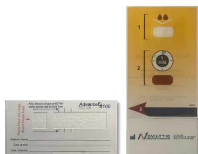
Fig. 1: Two types of DBS cards. Left card produces ~30 \mu L of serum; right produces ~6 \mu L serum.
